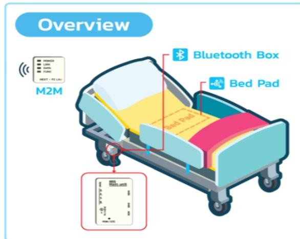
**Figure 1.** Composition of the bed sensor equipment provided in MIMAMORI system
