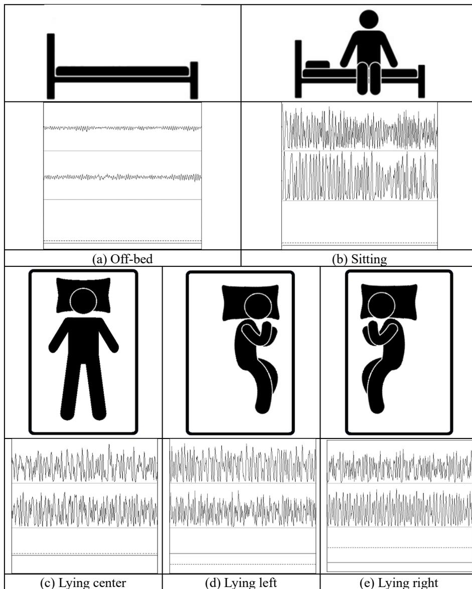
**Figure 5.** Correlation between signals and positions, where the first solid line is the signal of piezoelectric sensor on the left, the second solid line is the signal of piezoelectric sensor on the right, solid line is the signal of FSR weight sensor on the left, and dash line is the signal of FSR weight sensor on the right
