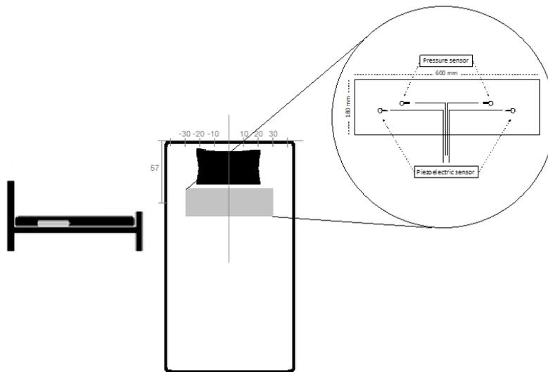
Figure 4. Placement of the bed sensor pad
