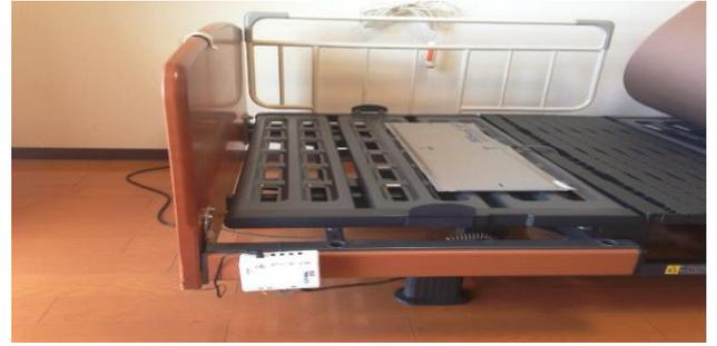
Fig. 1. Position of sensor panel on the bed
